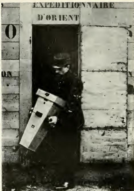
Apparatus used by the French for taking photographs from *aéroplanes*.
