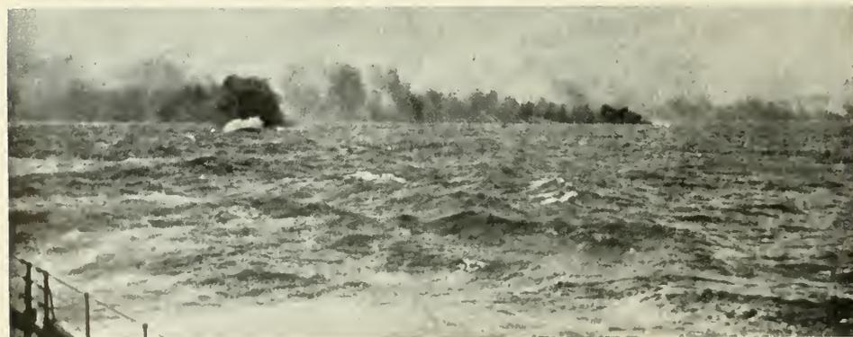
Smoke screen evolutions. *Torpedo boat destroyers practising screening of convoy by means of smoke, which is given off by the oil burners under the boilers.*
